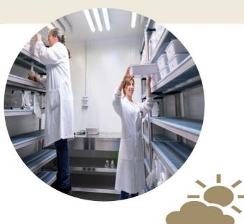
Two environmental chambers for mosquitoes rearing in small and medium size cages
